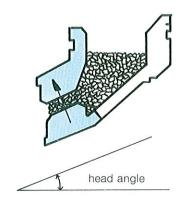
Gyradisc liners are shorter and less inclined than conventional cone crusher liners. Their method of fixing enables quick and easy replacement and eliminates the need for backing material.
