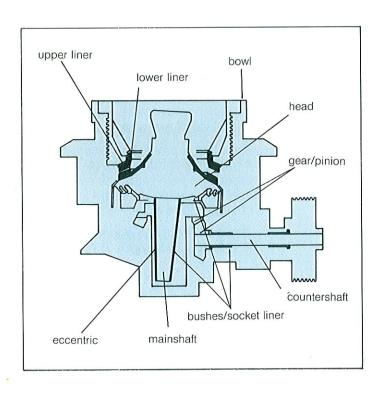
The major components of the Gyradisc are illustrated (left) in this cross sectional view.
