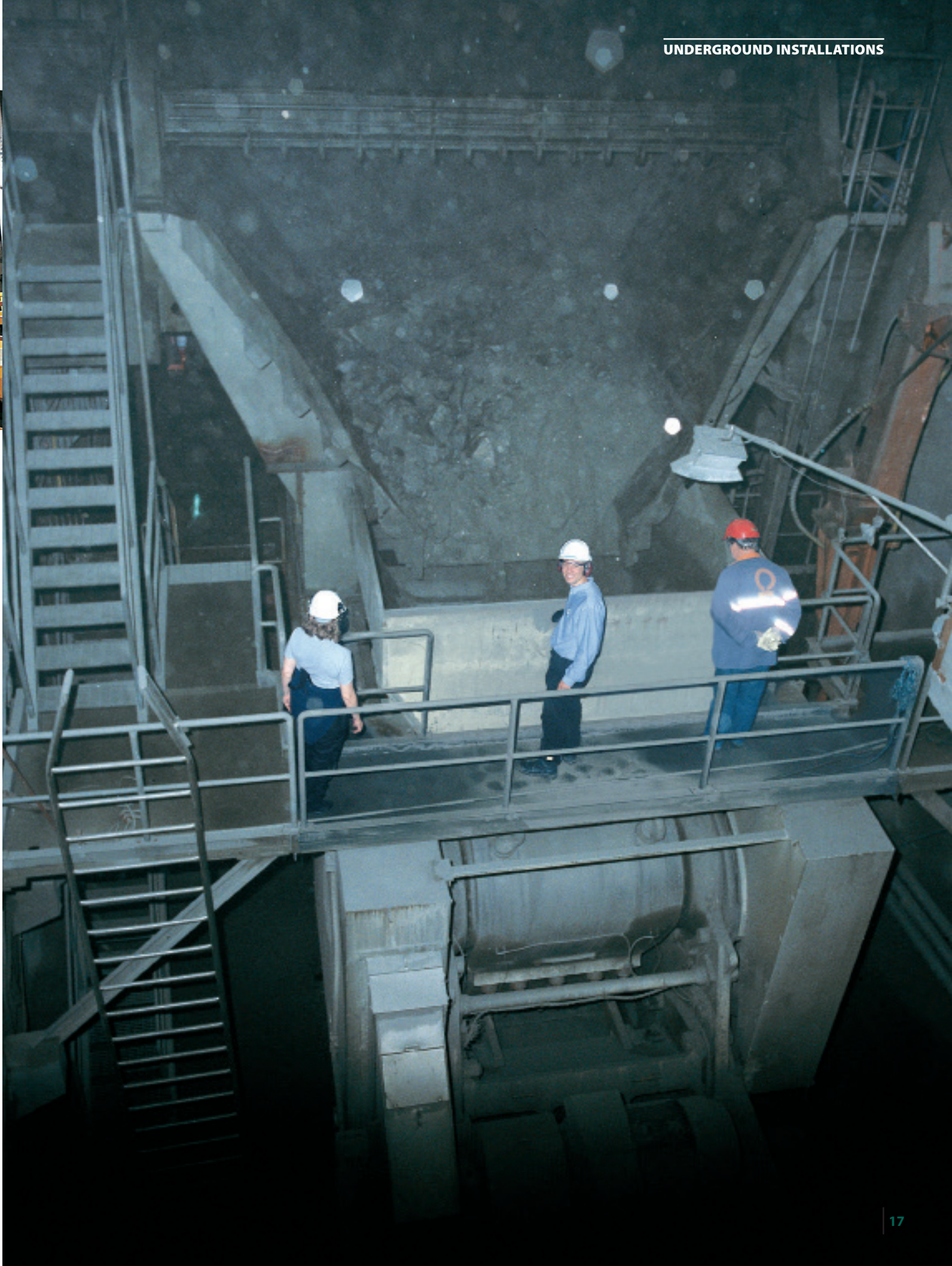
C200 in operation in a zinc and copper underground mine 1400 meters below ground. The crusher is monitored and operated from the surface control room.
