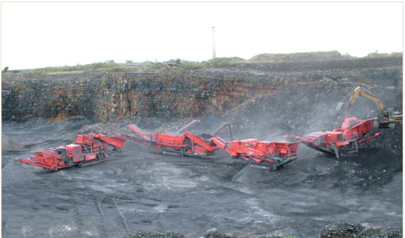
J-1480 Jaw Crusher, I-130 Impact Crusher, 984 Horizontal Screen and C-1540RS working in sequence
